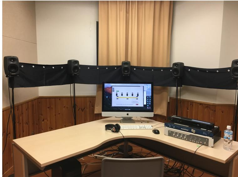
Fig. 3.4 Setup of subjective listening experiment
