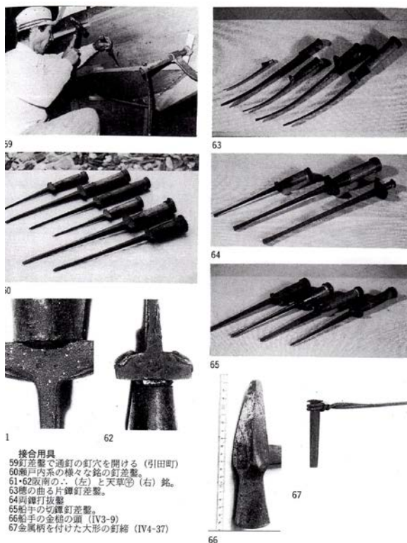
Fig.6 Comparison of the shape of the Funa-kugi and Tuba-nomi. 28)
