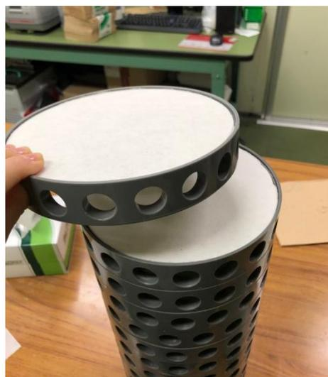
Fig. 1-8 Drying in the constant-temperature and constant-humidity chamber
