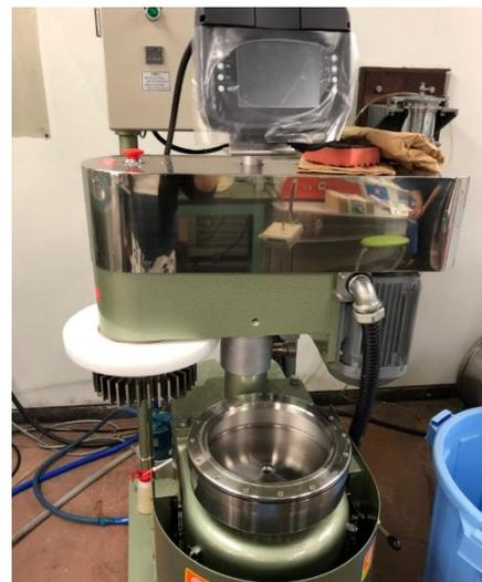
Fig. 1-4 Beating of pulp by using PFI mill
